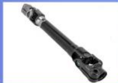
Steering Column Shaft
